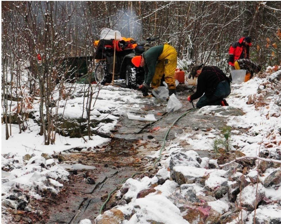
Figure 8: Technicians Putting Rock Samples in Appropriate Bags
